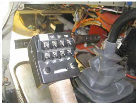
Figure 18 - The switches in Bell 412 helicopter which will be used in the detection and discrimination process.
